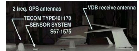
VDB and GPS antennas (sensor system) on roof of A/C
