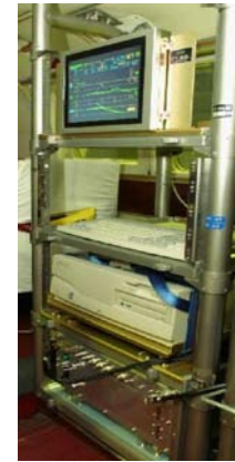
VDB receiver and GBAS A/C data processor
